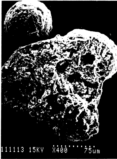
Figure 1. SEM view of an FCC catalyst particle (Reproduced with permission. Copyright 1993 Institution of Chemical Engineers.)
